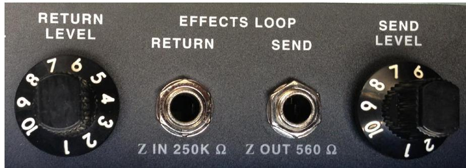
**Effects loop picture 55watt version shown** (25watt version has in and out but no level controls)
